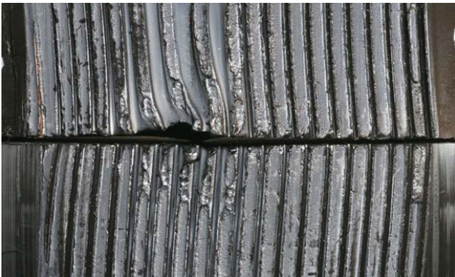
Figure 9: Ductile fracture (tearing) of the PE between the windings
