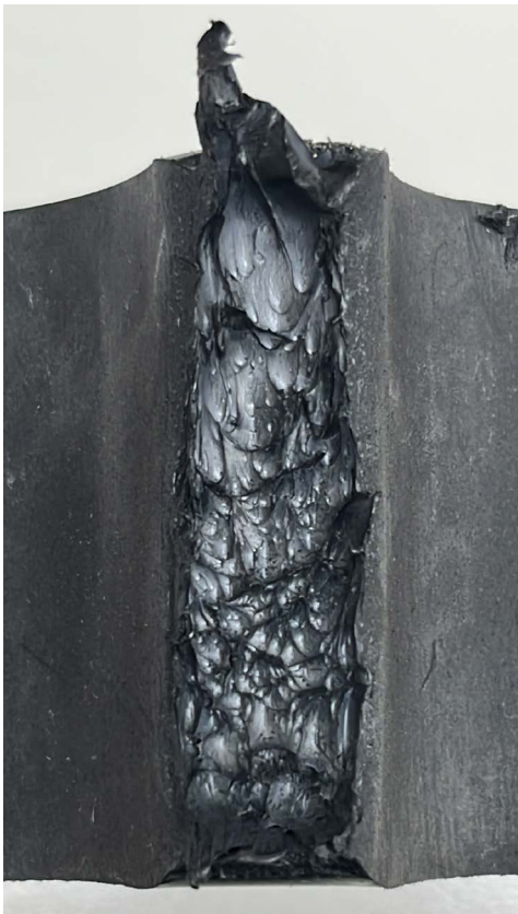
Figure 2: DN800 SDR11 Ductile failure mode photo with corresponding stress vs extension graph.
