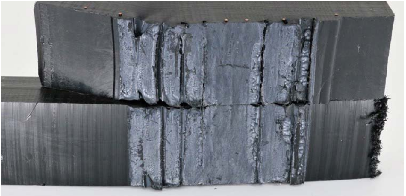
Figure 11: shows a large brittle area of brittle separation at the interface of the pipe and fittings surface
