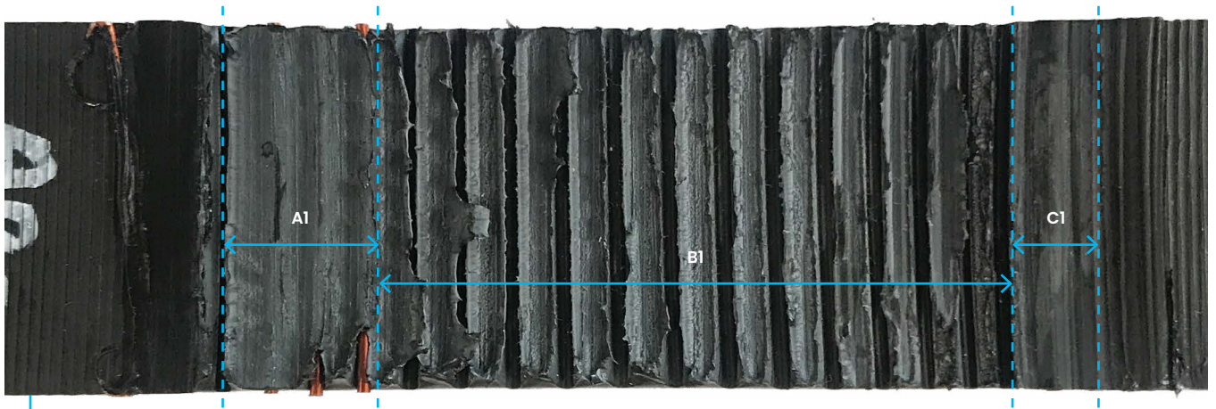
Figure E1.1: Electrofusion coupler – plan view of full fracture zone based on the close-up image shown in Figure 11.
