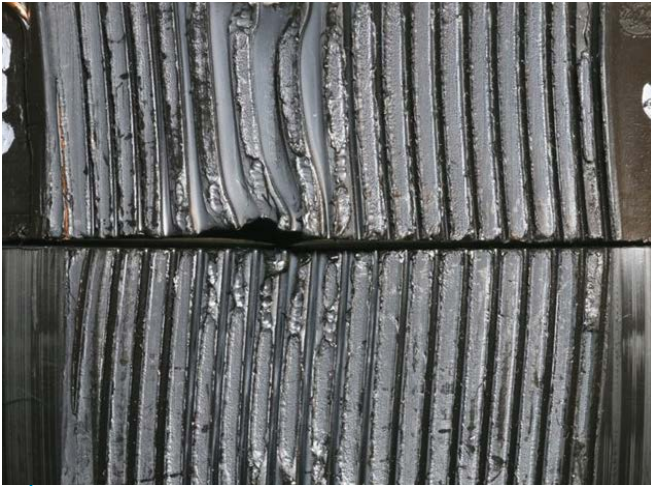
Figure 5 – shows ductile fracture (tearing) of the PE between the windings. Stress whitening is apparent across most of the fusion zone surfaces, with some gross ductility near the edges towards the centre of the test piece. This is a Pass result.
