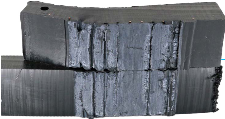
Figure 7 – shows a large area of brittle separation at the interface of the pipe and fitting surfaces. This is a Fail result.
