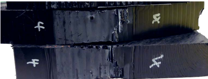
Figure 10 – shows brittle separation at the interface by the featureless surface. This is a Fail result.
