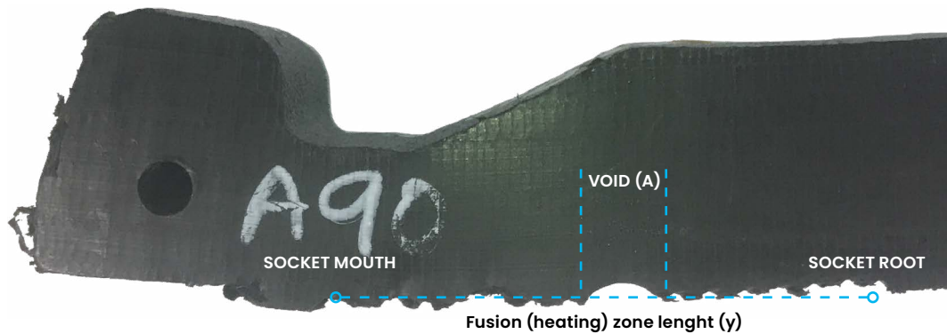
Figure E2.2: Electrofusion coupler – side view of the full fracture zone.
