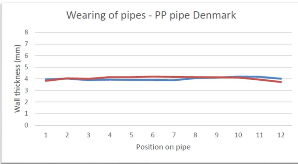
Position 1 is the upper part of the pipe, and position 7 is the lower part of the pipe and therefore the area where the main flow of the storm water runs. DTI concluded on basis of the measurements that: "The wear of the wall thickness is too minuscule to be measured with normal gauge used for measuring wall thickness. No wear could be detected."
