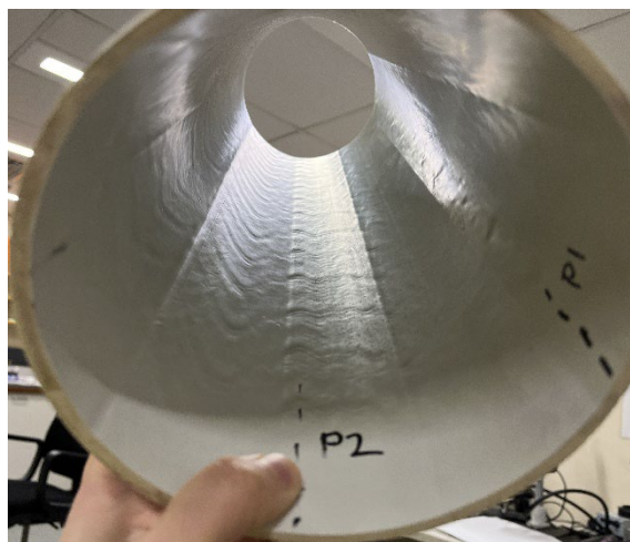
Figure 4: The same section of DN150 DWV bore rippling, photo taken in laboratory with phone camera.
