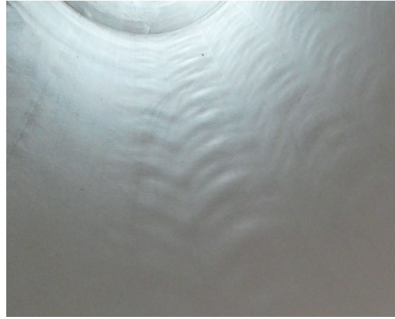
Figure 6: DN225 DWV bore rippling – view 2 photographed by phone camera.
