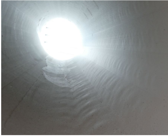
Figure 5: DN225 DWV bore rippling – view 1 photographed by phone camera.
