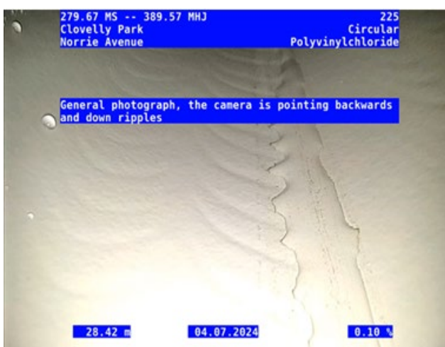
Figure 2: DN225 DWV bore rippling – CCTV view 2.
