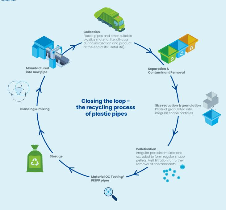
Plastic pipes like PVC can be recycled mechanically 8 to 10 times without loosing their technical properties. Assuming a pipe lifetime of 100 years, this plastic pipe material may have a lifetime exceeding 800-1000 years.
