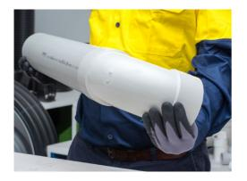
Hold the joint against movement and rejection (i.e., pushback) of the spigot for a minimum of 30 seconds.
