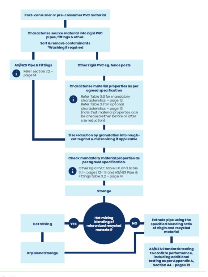
**PIPA POP208 -** Specification and testing guidelines for recycled materials suitable for non-pressure plastic pipe applications. Polyethylene, Polypropylene and Rigid PVC - Issue 1.0 June 2022
