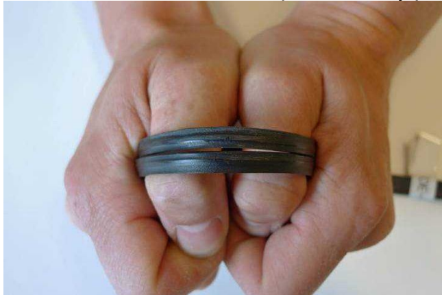
Figure 5: Bead Bend Back Test. The beads separate indicating a bad fusion.
