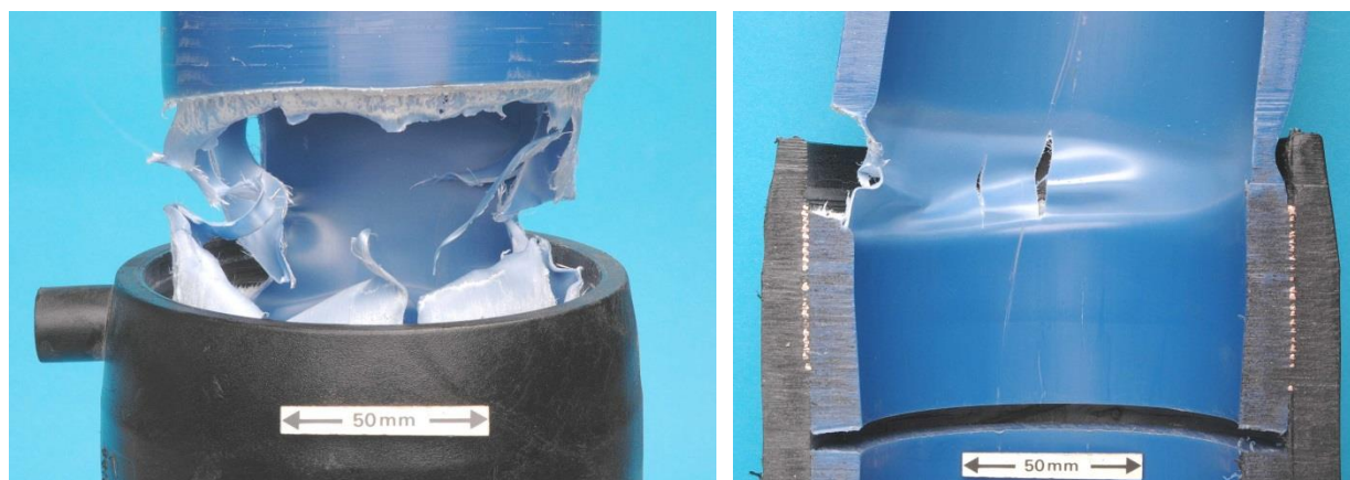
Figure 5: Typical failure of an unflawed EF joint in PE pipe when subjected to a constant tensile load at elevated temperature, showing failure initiating from the external cold zone notch between the pipe and fitting.
