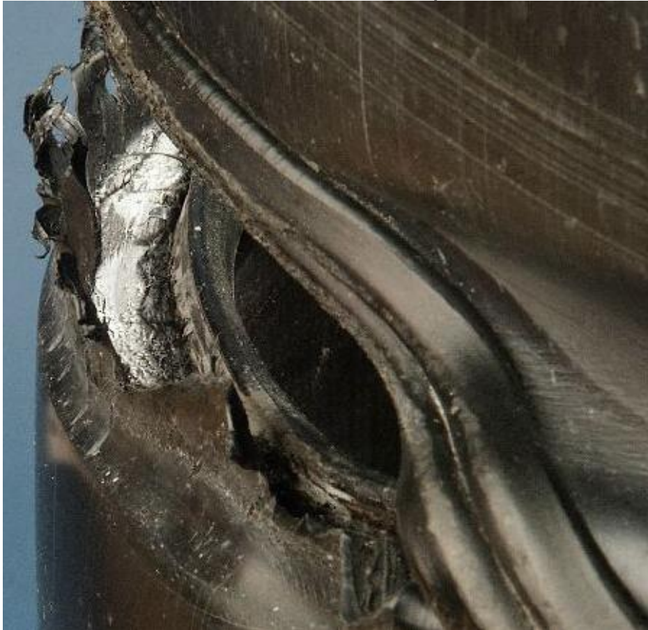
Figure 3: Typical failure of an unflawed butt fusion joint in PE pipe when subjected to a constant tensile load at elevated temperature, showing failure initiating from the notch between the weld bead and the pipe wall.
