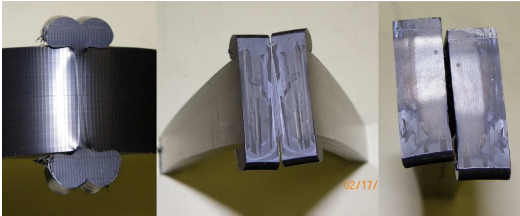
Figure 8 - Bend test results on pipe joint 1224 (standard fusion procedure), left two images, and on pipe joint 127 (worst fusion condition) on the right
