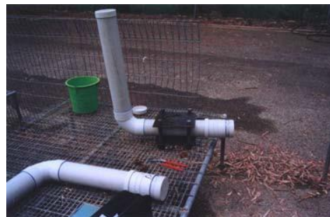
FIG.2 HORIZONTAL ASSEMBLIES. ONE WITH 7.5% DEFLECTION APPLIED TO THE SPIGOT VIA 2 PARALLEL STEEL PLATES
