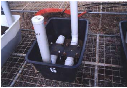
FIG. 3 TWO HORIZONTAL ASSEMBLIES WITH 7.5% DEFLECTION APPLIED AND READY FOR BURIAL
