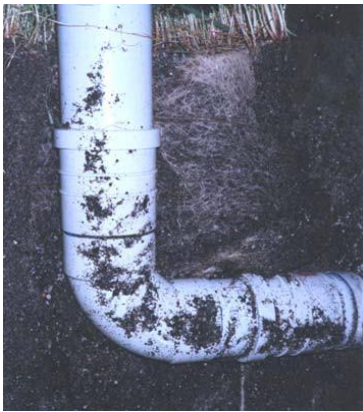
FIG. 6 RYE GRASS ROOTS BINDING ALL THE SOIL TOGETHER, INCLUDING THAT BELOW THE ASSEMBLY
