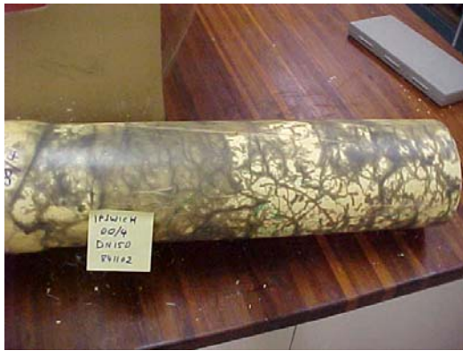
Figure 5. Typical external staining pattern. Figure 6. Wall thickness of individual pipes.
