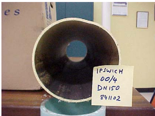
Figure 3. Distortion in spigot of 00/4.
