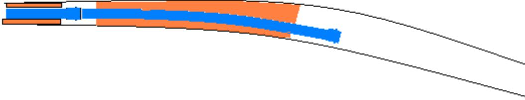
3. Bending of pipes is achieved after each joint is made, by laterally loading the pipe. The techniques used to load the pipe to achieve the curve will vary dependent on pipe size, class and type as clearly the forces required to induce bending vary over a very large range.
