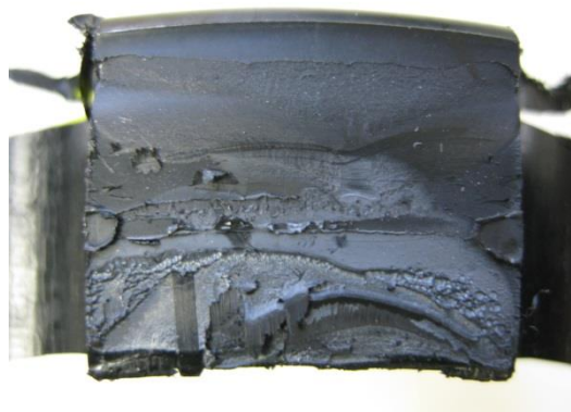
Figure 3: showing "mixed" and brittle failure modes of tensile specimens.
