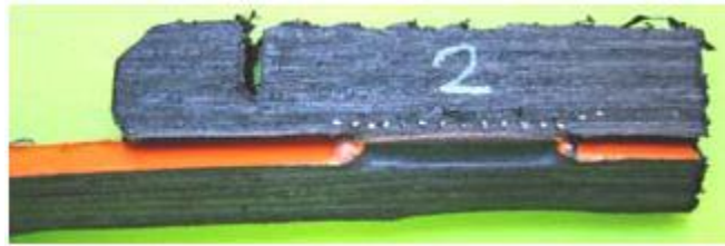
Figure 7: ISO 21751 strip bend test showing acceptable EF weld after bend testing.
