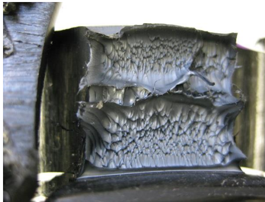
Figure 2: showing fully ductile failure mode of tensile weld specimens.
